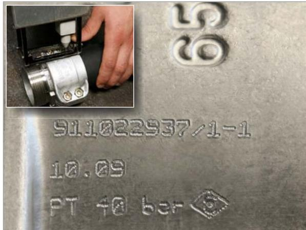
Coding of Hose Assembly on Spannloc Fitting
